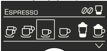
The status line **5a** in the display **5** shows the name of the type of drink, along with the strength setting, e.g.  $\text{00}$  and per-cup quantity, e.g.  $\square$ . The selection line **5b** shows symbols for drink selection.
